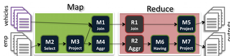
Figure 5.8: Single MR-LEGOS job definition for the two SQL queries shown in Figure 5.6.
